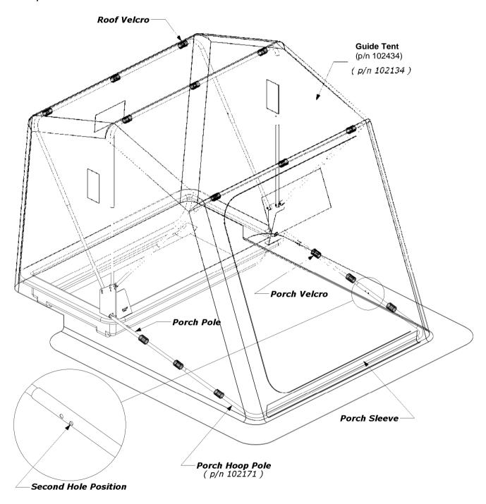
To "set" the tent, grasp the tent material at the rear of the shelter and pull it downward. Observe the porch area of the tent lifting accordingly as you pull. When the U-Channel molding is correctly installed, the porch hoop pole will lightly touch the floor.
